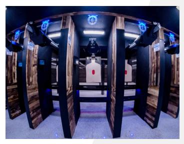
users can manage static paper targets, as well as dynamic paper targets, to automatically turn 360 degrees during friend and foe scenarios.
