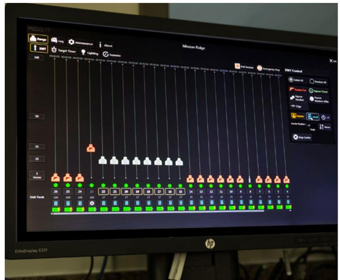
The **XWT Lane Manager** allows the range operator to control the lane from any browser on the InVeris network. It also:
